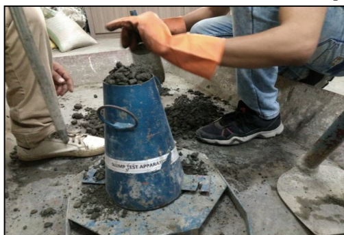
Fig 3.13 Slump Cone Test 1/4
