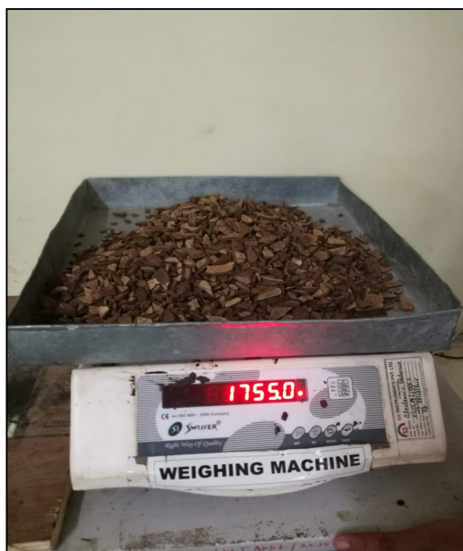
Fig 3.10 Weighing oven-dried coconut shells
