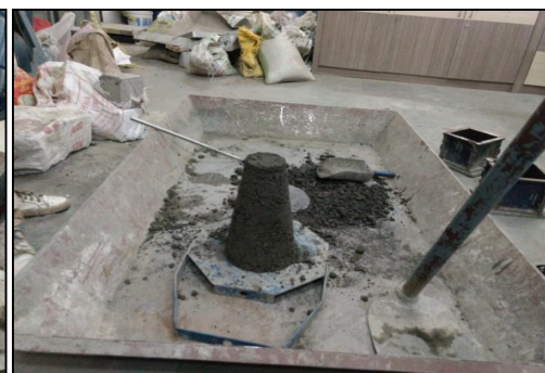
Fig 3.14 Slump Cone Test 2/4
