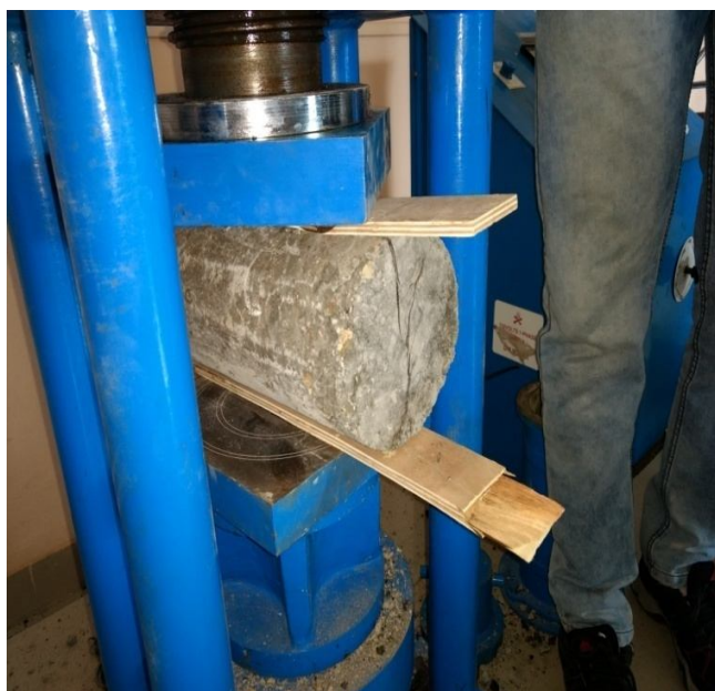
Fig.3.28 Testing cylindrical concrete specimen
