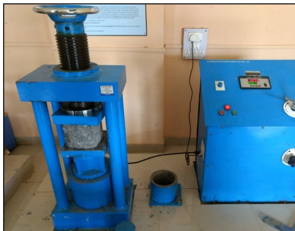
Fig 3.20 Compression Testing of cubes
