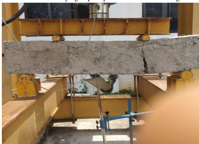
Fig. 11 crack in the specimen
