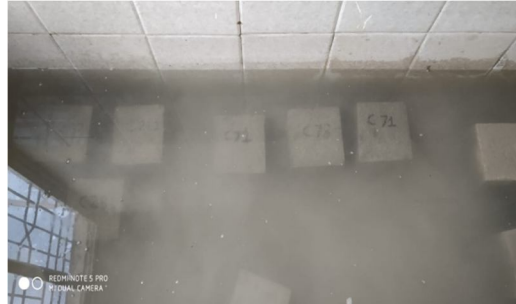
Fig. 4 Curing of Cubes
