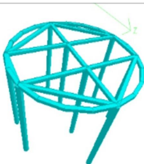
Hexagonal Cross Bracing
