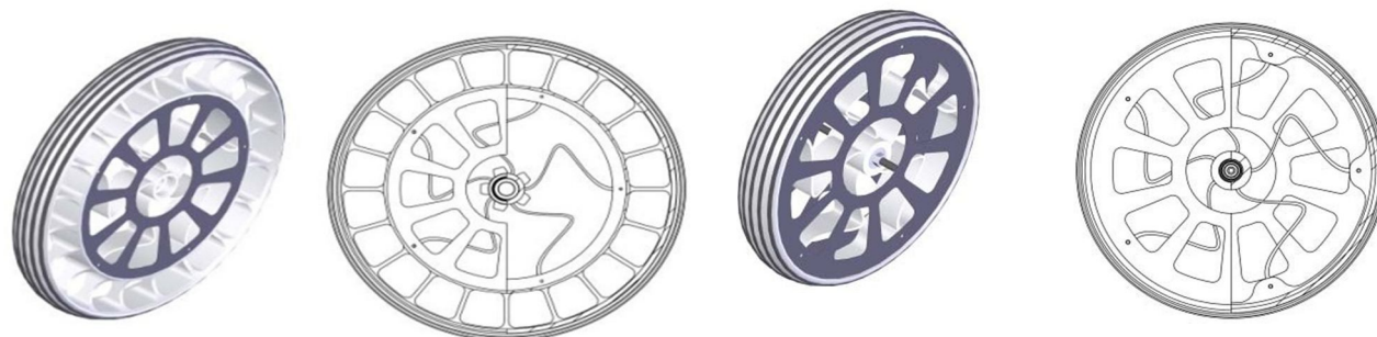
Figure 4.5 - Fixed joint IWS design for baby stroller; Left: front wheel Right: rear wheel
