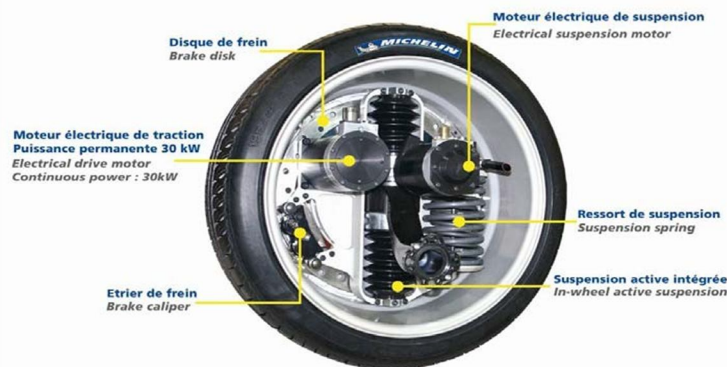
Figure 2.3 - Michelin active wheel (Michelin re-invents the wheel, 2008)
