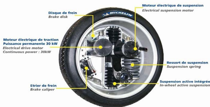
Figure 2.3 - Michelin active wheel (Michelin re-invents the wheel, 2008)
