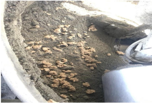
Figure 3: Mixing the constituent materials with Grinded Cigarette Butts
