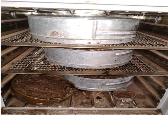
Figure 1: Oven Drying of Cigarette Butts at 150°C
