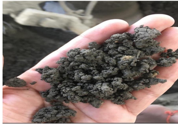
Figure 4: Cellulose Acetate fibers mixed with the constituent materials
