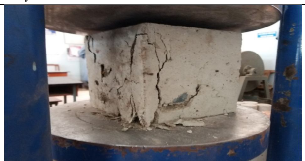
Compressive Strength test (CTM equipment)
