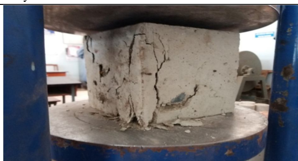
Compressive Strength test (CTM equipment)
