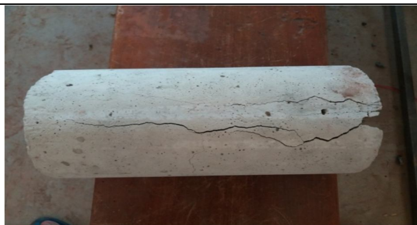
Cracked formed in cylinder after applying load
