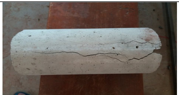
Cracked formed in cylinder after applying load
