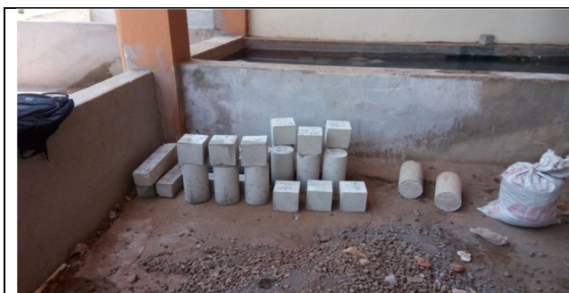
Concrete Cubes, Beams and Cylinder casted and ready for curing in curing tank
