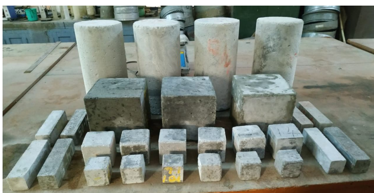
Fig. 1 Different size of mortar specimens casted
