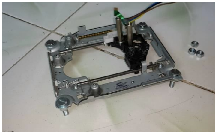
Required Part of CD-ROM along with stepper motor
