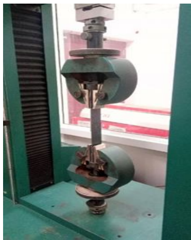
Fig 3.2 Tensile test conducting on Tinius Olsen machine
