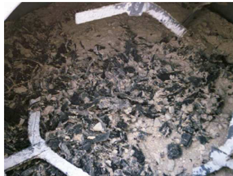
Fig. 5. Preparation of rubcrete mixtures.
