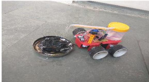
Figure 4: Robot extinguishing fire.
