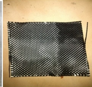
Fig.2: Preparation of Carbon Mat
