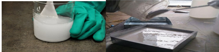
Fig.3: Preparation of Epoxy Resin and pouring to the mould
