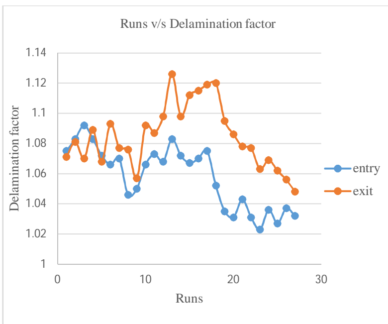
Fig 7 Graphical representation of entry and exit of delamination factor for CFRP with different percentage of Si 3 N 4
