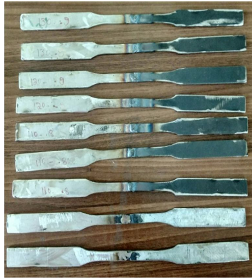
Figure 4: prepared specimen after machining
