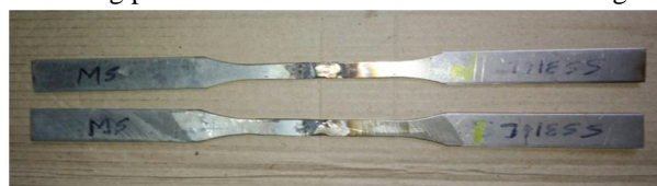
Figure: 2 dissimilar materials welded using TIG welding
