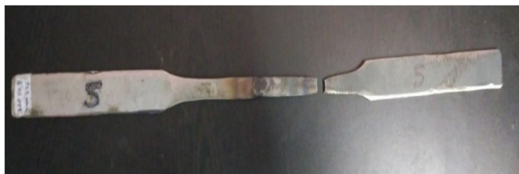
Figure 7: Specimen after Tensile Test
