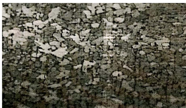
Figure 16 : Microstructure of Parent Zone 500X
