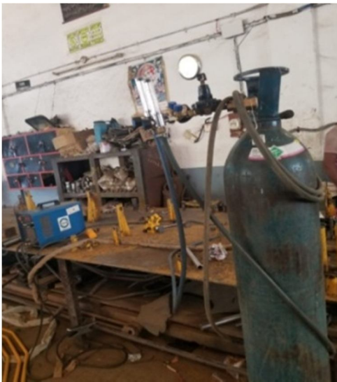
Figure 3: Experimental set up of TIG Welding
