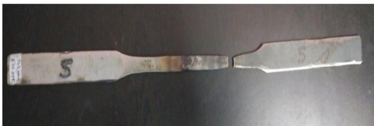
Figure 7: Specimen after Tensile Test
