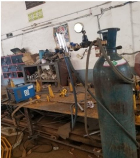
Figure 3: Experimental set up of TIG Welding
