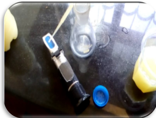
Plate 3.4 TSS Determination using Refractometer
