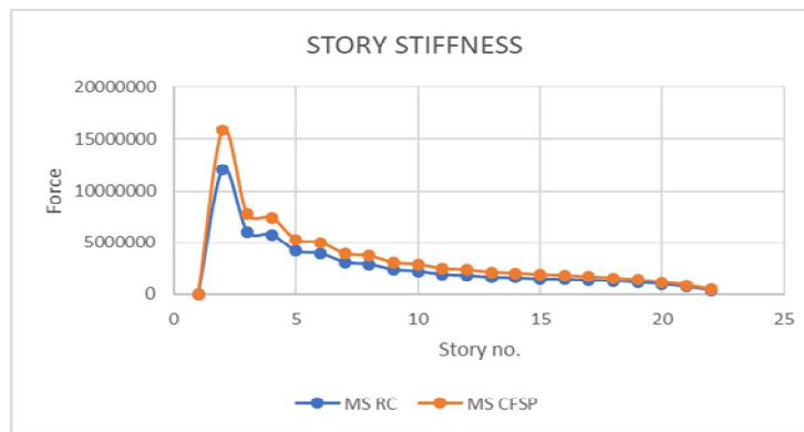
Fig 11: Storey Stiffness of RC Diagrid and CFST diagrid structures in Medium soil
