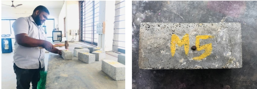
Figure. 5 Nailing Test on Bricks
