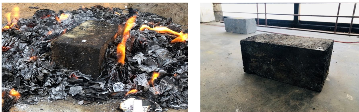
Figure. 7 Fire Test On Brick
