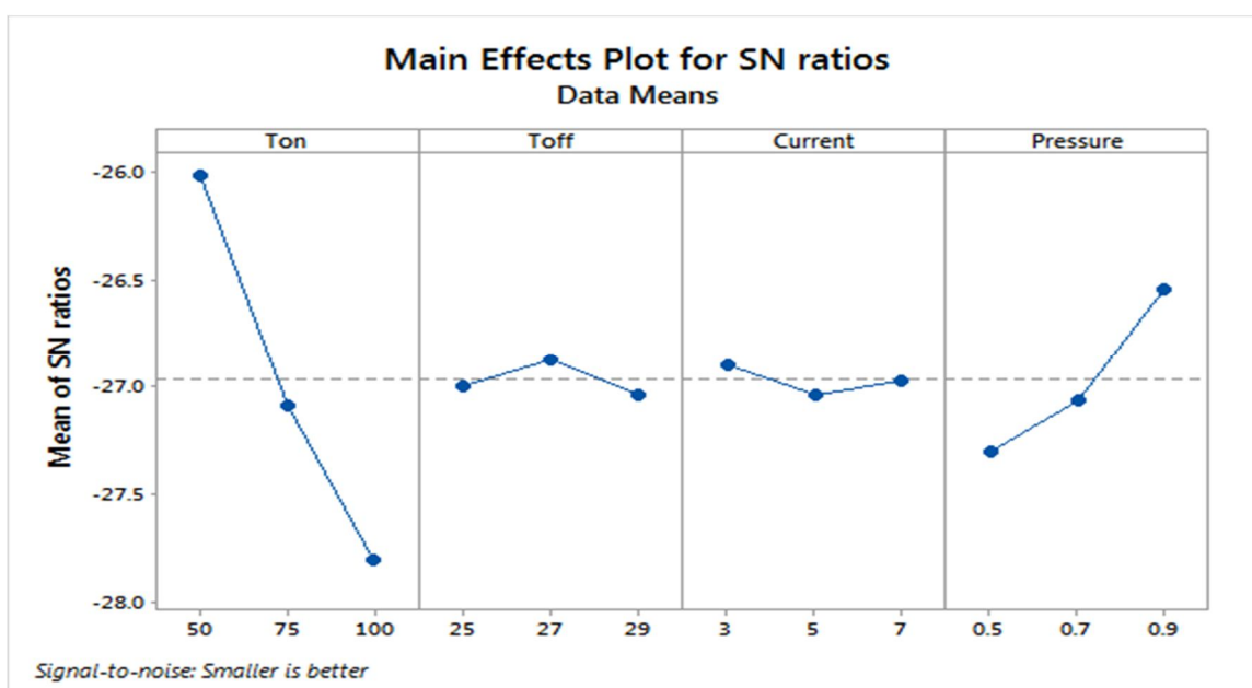
Signal To Noise ratio analysis for Pentagonal Cut for OC
