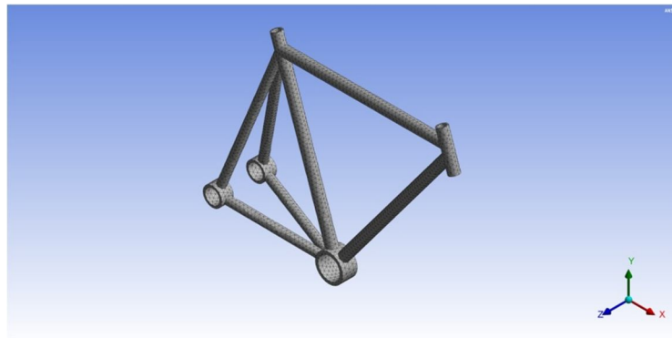
Fig. 3 Bike frame with meshing of 5mm
