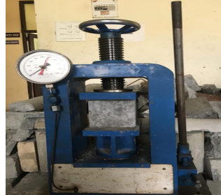
Compression test of cube
