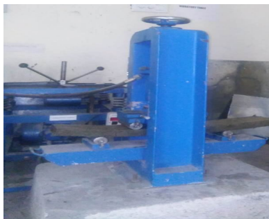
Testing of Flexural strength of slab
