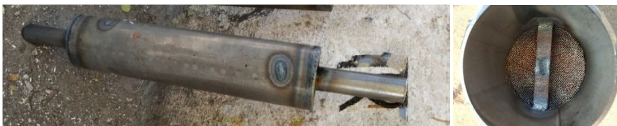
Figure 3. Actual Model of Catalytic converter
