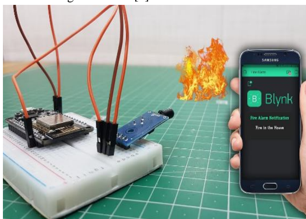
Figure.8 Blynk App for Smart Smoke Alarm
