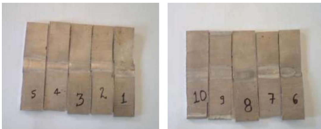
Figure 1: Welded specimen performed with (a) welding speed 3.50 mm/s and welding current 100, 110, 120, 130 and 140 A for sample no 1, 2, 3, 4, 5 respectively (b) welding speed 4 mm/s and welding current 100, 110, 120, 130 and 140 A for sample no. 6, 7, 8, 9, 10 respective.
