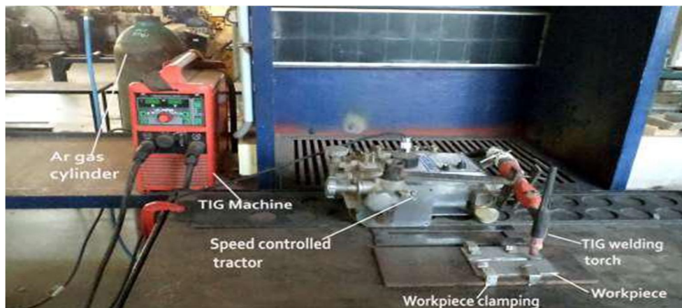
Fig. 1:- Mechanized TIG welding setup
