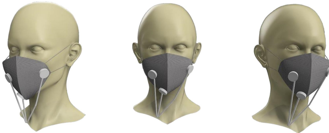
Fig. 3 special design mask with muscle/emg sensor
