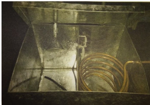
Fig. 2. fabrication of humidification and de-humidification Chamber with GI steel
