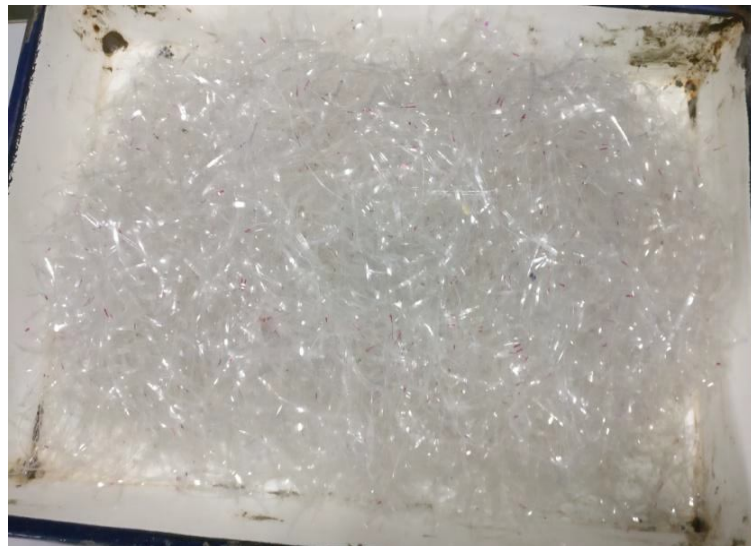
Fig. 1 Fibers of aspect ratio 50mm x 2mm
