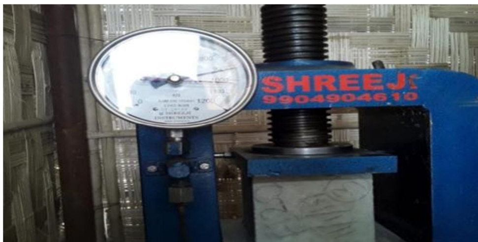
Figure 3: Cube testing for getting Compressive strength of sampl
