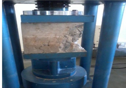
Figure 3 Crushing strength test
