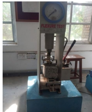
Figure 4 Flexural Strength Test Apparatus
