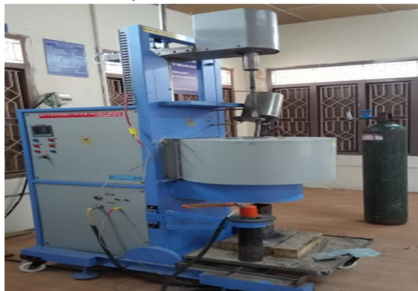
Fig.5. Bottom type Stir casting equipment
