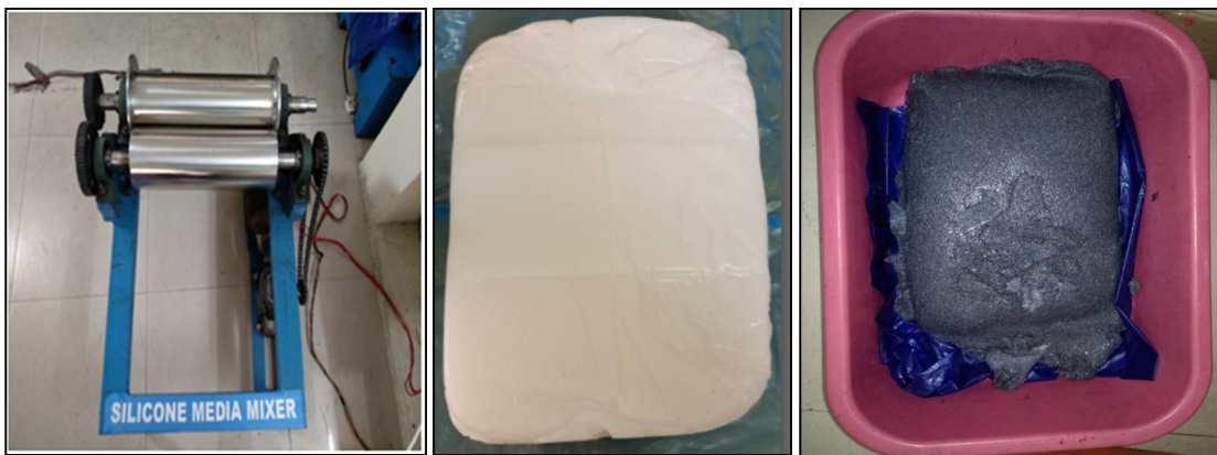
Fig 3(a): Silicon media mixer Figure 3 (b) Silicon Rubber Figure 3 (c): Silicon polymer with abrasive
