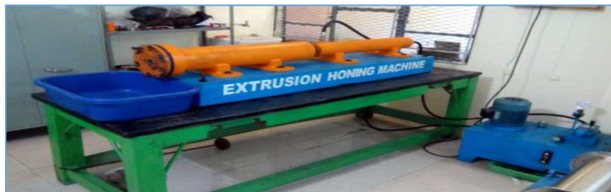
Fig 1: one way type of extrusion honing Machine
