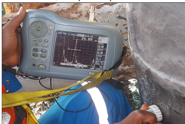
Figure -1: Ultrasonic Testing on cracks
