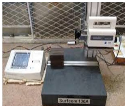
Fig 2.4: Surface roughness measuring instrument (Surfcom 130A)
