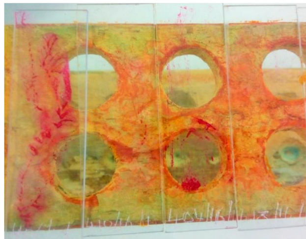
Smearing and staining of Glass Slides with Eosin Reagent
