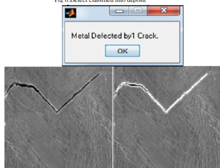
Fig. 7. Defect classified into crack
