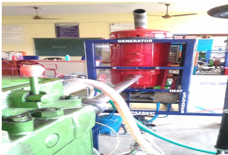
Fig.1: Generator is connected to engine exhaust manifold pipe
