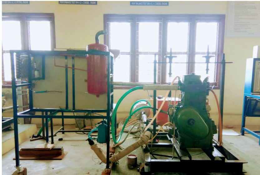
Fig.2: Experimental setup on VAR system is connected to the diesel engine
