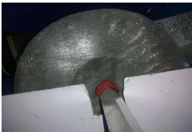
Fig 3.: Film formation on the mesh disc
