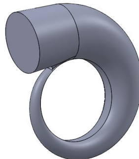
Fig. 3 3D CAD models of the volute casing
