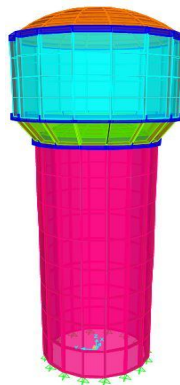
Fig. 1 Elevated Water Tank Model in SAP2000
