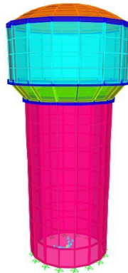
Fig. 1 Elevated Water Tank Model in SAP2000
