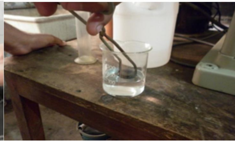
Fig. 8 Specimen Etching Process
