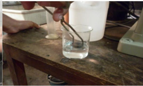
Fig. 8 Specimen Etching Process
