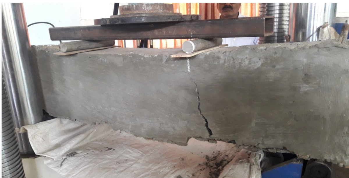
Figure-13 Crack width of control beam.
