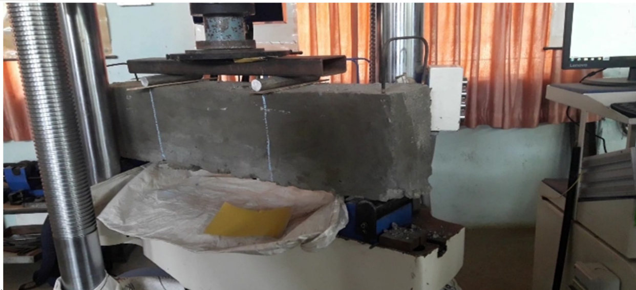
Figure-14 CFRP R.C deep beam before testing
