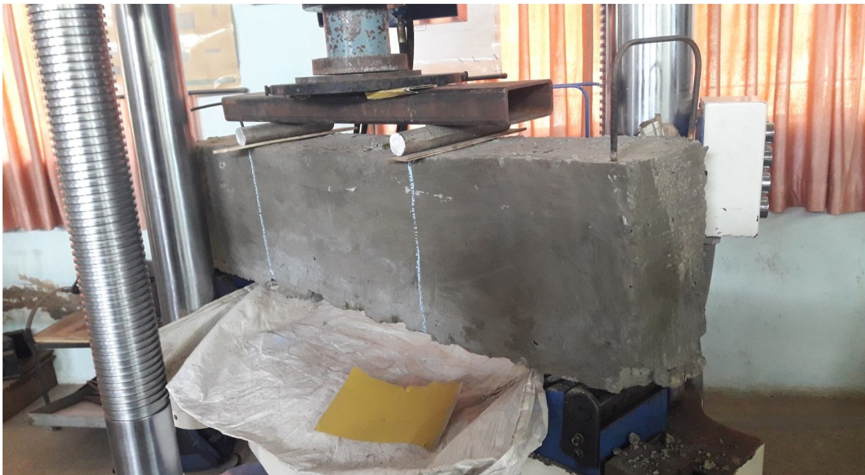
Figure-4. Two point loading test set-up.
