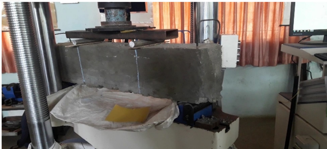
Figure-14 CFRP R.C deep beam before testing
