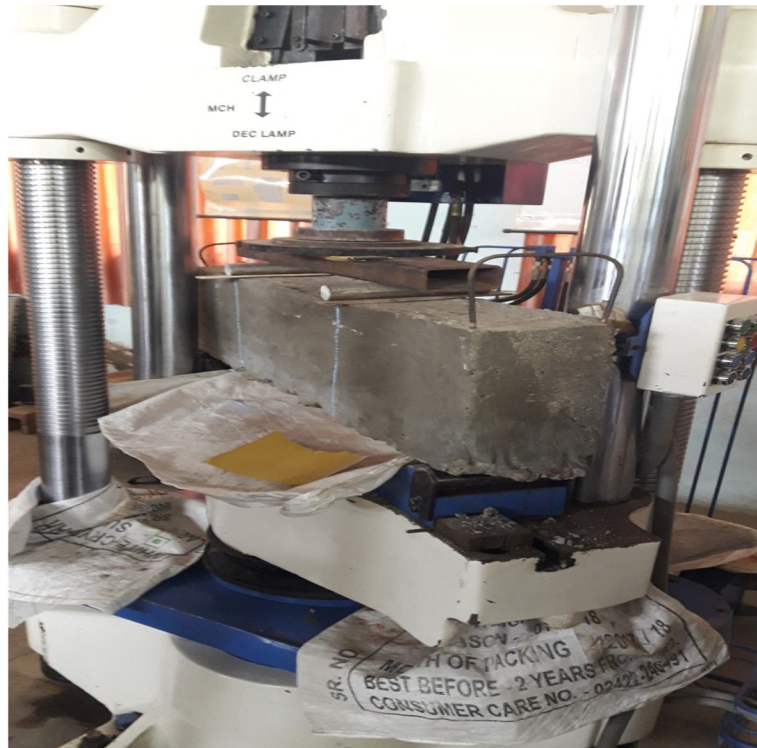
Figure-7. Test beam fixed on UTM assembly.
