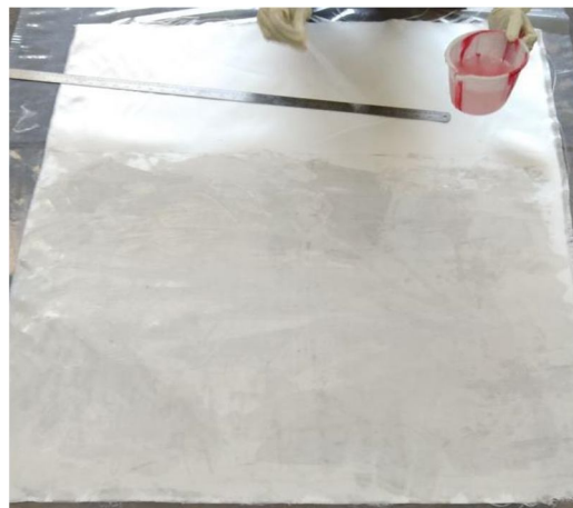
Fig.12. E-glass Fabric with Epoxy Resin Hand Layup
