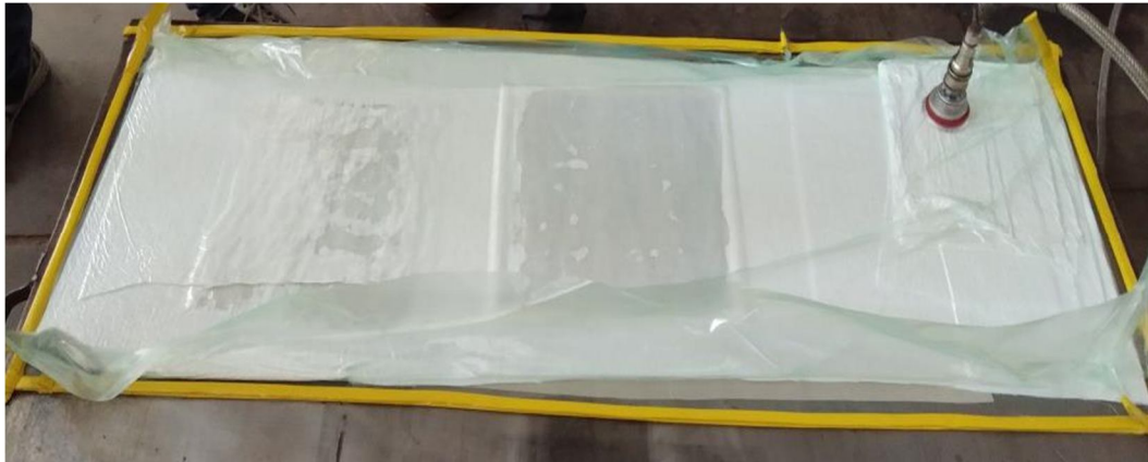
Fig.14 Vacuum Bagging of Laminate
