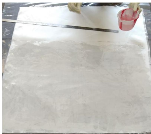
Fig.12. E-glass Fabric with Epoxy Resin Hand Layup
