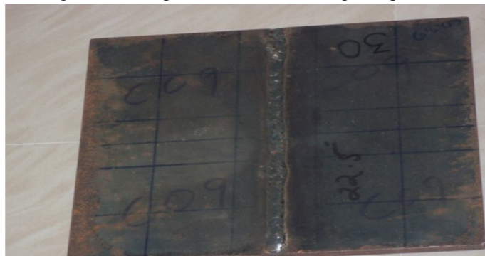
Figure3. Weld plate after welding by CO 2 arc welding process
