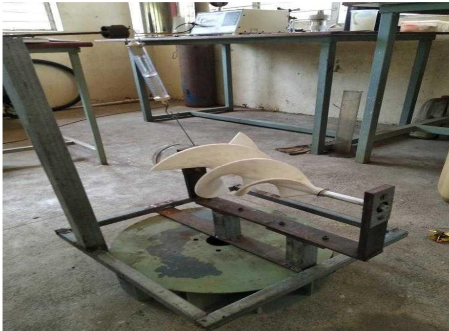
Figure 4 Experimental set up of wind turbine model assembly
