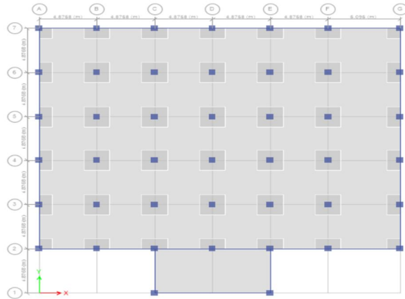
Figure 1: Plan View of Flat Slab Structure
