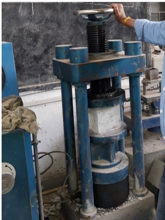
Fig.2. compressive strength test on CTM Machine
