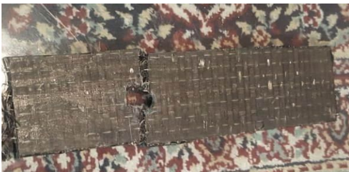
Fig. No. 30: Plate 1 after tensile test
