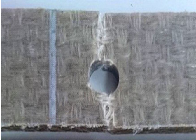
Fig. No. 32: Plate 2 after tensile test
