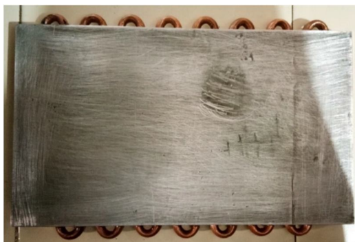
Fig. 3.2. Perforated block heat exchanger (fabricated)
