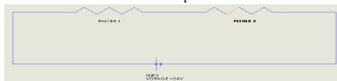
Fig. 3.14. Schematic of series connection
