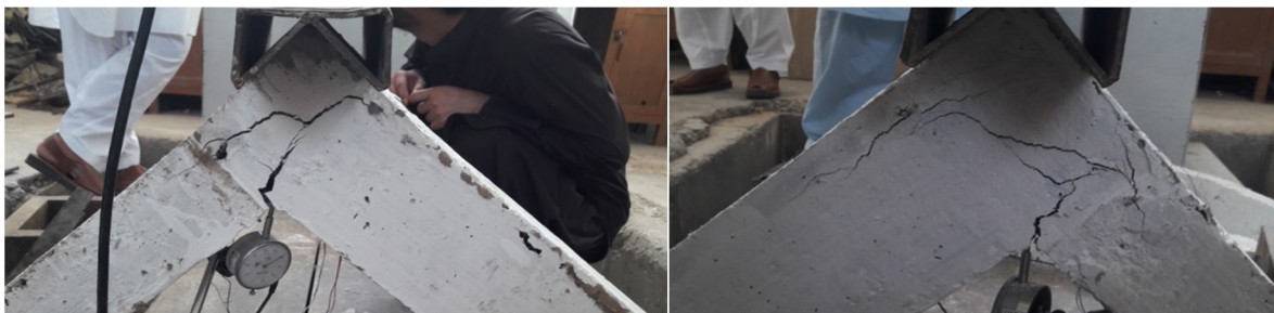
Figure 4.1: Cracks development in the conventional concrete (left) and ECC (right).
