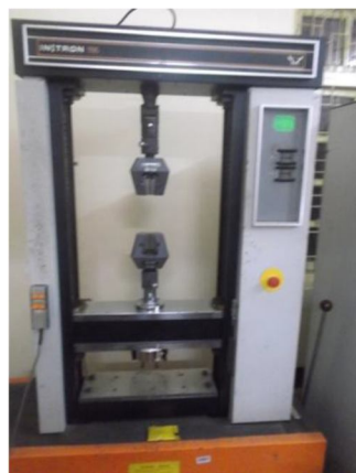
Fig: 3.2 a. Experimental set up of tensile test
