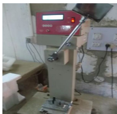
d. Experimental setup of impact test
