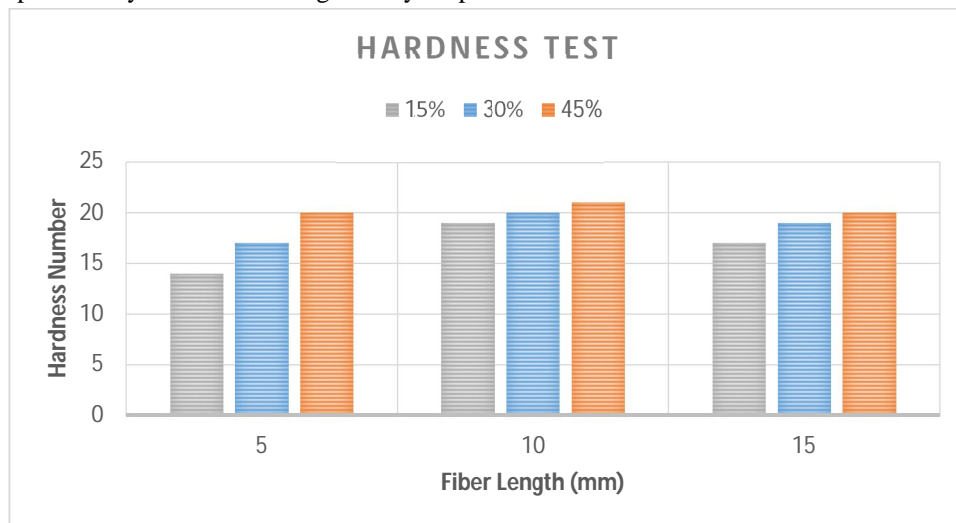
Figure 4.4 Hardness Properties for Bamboo Fiber reinforced composites
