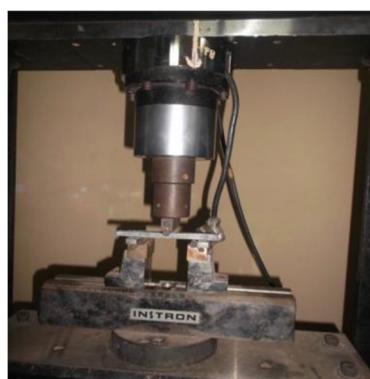
c. Loading arrangement for flexural test
