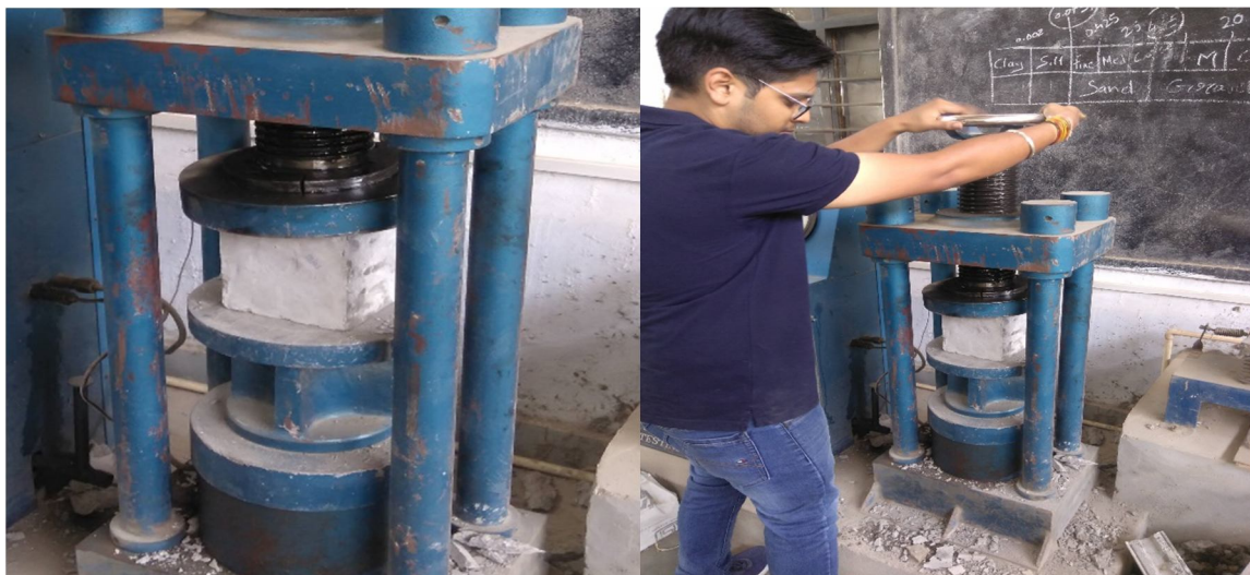
Fig. 3 Concrete cube under compression testing.
